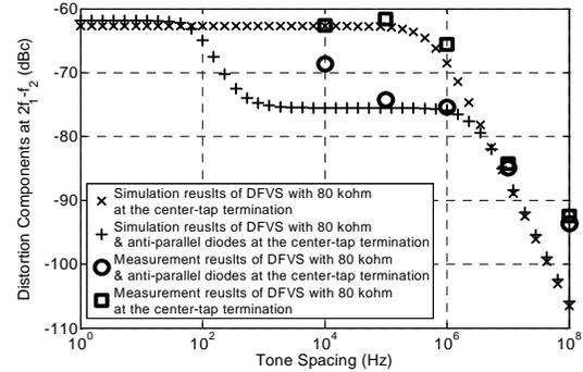
Fig. 4. Simulated and measured distortion component at  $2f_2 - f_1$  as function of tone spacing at a power level of 18 dBm for the DFVS making use of TU Delft in-house silicon-on-glass technology ( $f_{center} = 2.14$  GHz,  $V_R = 5$  V and  $C_{j0} = 2.3$  pF) [13].
