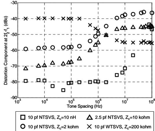
Fig. 8. Measured distortion component at  $2f_2-f_1$  as function of tone spacing at a power level of 20 dBm for the WTSVS and NTSVS making use of Skyworks’ GaAs technology (for all cases:  $f_{center} = 2 \text{ GHz}$ ,  $a_2 = 0.183 \text{ V}^{-1}$  and  $V_R = 5 \text{ V}$ ).
