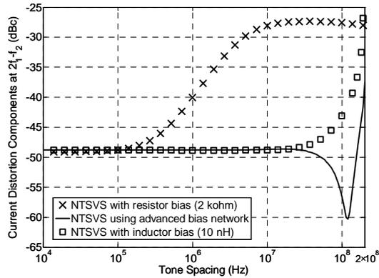
Fig. 7. Simulated capacitive current distortion component at  $2f_1-f_2$  versus the tone spacing of the input RF voltage signal ( $a_2=0.183 \text{ V}^{-1}$ ,  $V_{R,max}=12 \text{ V}$ ,  $V_R=5 \text{ V}$ ,  $V_{RF,peak}=10 \text{ V}$ ,  $f_{RF,center}=2 \text{ GHz}$  and effective capacitance at zero bias=10 pF) for the NTSVS with different center-tap networks.
