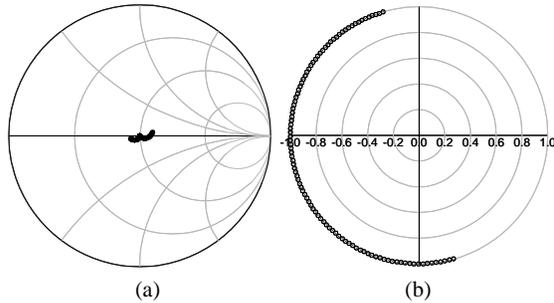
Fig. 10. (a) The simulated  $s_{11}$  of the fictive phase shifter (b) Polar plot of the simulated  $s_{21}$ . [The lossless series inductances ( $L_{series}$ ) in Fig. 9 are fixed as 0.36 nH, while the shunt capacitances ( $C_{shunt}$ ) are tuned from 7.35 pF to 13.60 pF. The characteristic impedance is  $5 \Omega$  and the RF frequency is 2 GHz].
