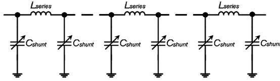
Fig. 9. Schematic of the true-time-delay phase shifter to be used for system-level linearity comparison for different varactor configurations. [To achieve a phase shift of  $180^\circ$ , eight  $\Pi$  low-pass sections are cascaded. The lossless series inductances ( $L_{series}$ ) are fixed as 0.36 nH, while the shunt capacitances ( $C_{shunt}$ ) are tuned from 7.35 pF to 13.60 pF. The characteristic impedance is  $5 \Omega$ .]
